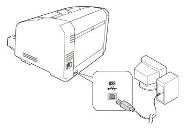
If the plug does not attach easily, make sure that you are plugging it in correctly. Do not force the plug into either connection.
