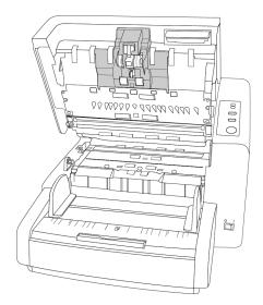
1. Pinch the sides of the paper feed roller cover and pull it towards you to access the rollers.
