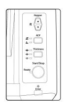
**Hopper**—the up and down arrows adjust the height of the input tray based on the amount of paper in the input tray. The scanner will automatically raise the tray during scanning, but if you regularly scan small batches of paper, you may want to keep the input tray higher to save time adjusting the height automatically while scanning.
