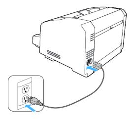
Note: Do not turn on the scanner until after you install the software.
