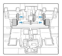
7. Lift the roller cover up and carefully push it closed to lock it in place. Make sure everything is aligned properly and the cover is fully closed. If the cover is not fully closed it will break during scanning and damage the scanner.
