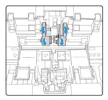
3. Pinch the plastic tab that locks the roller to the metal bar and pull the roller away from the bar. Do this for each of the rollers.
