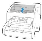
2. Release the retaining screw and then close the Pre-Imprinter door.
