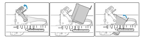
6. Lower the arms on the carriage to lock the ink cartridge in place.
