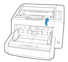
When you are done replacing the rollers, close the scanner carefully pressing down on both sides of the cover until it locks in place. Do not slam down the cover.
