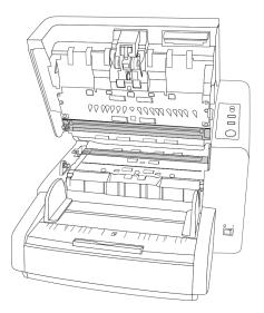
4. There is a green lever attached to each background plate. The sticker on each lever indicates which way to push the lever to change between the black and white background.
