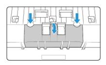
2. Lift the roller up and out of the scanner.
