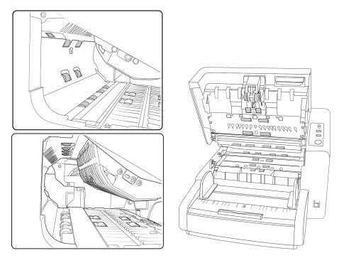
**Note:** Be careful when cleaning the rollers. All of the rollers, except the free rollers, are designed to rotate in one direction only. Do NOT force the roller to rotate in the opposite direction. Forcing the roller to rotate will damage it, and cause the scanner to feed pages incorrectly.
