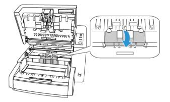
5. Align the roller bar with the brackets in the roller compartment. Make sure the groove on the right side of the roller bar is aligned so that it slides in place into the U shape of the bracket.
