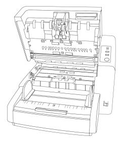
3. Point the tip of the blower at the sensor and squeeze the blower to direct a puff of air at the sensor head to remove dust.
