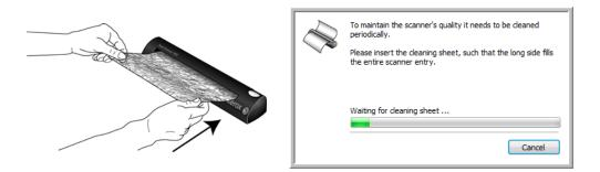
5. When the calibration or cleaning process is finished, the scanner will exit the page from the scanner. Remove the page after the scanner has released it.
