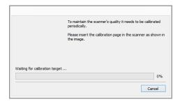
4. Place the calibration page in the scanner as shown in the following image.
