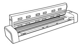
3. Gently close the scanner lid. Press down on both sides of the lid until you hear a click as the arms lock the scanner lid in place.
