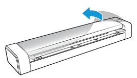
3. Place your thumbs on either side of the paper feed slot, underneath the lid of the scanner. Hold the scanner sides firmly and pull the scanner lid up to release it from the body of the scanner.
