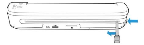
5. When you are finished cleaning the scanner, release the button on the side of the scanner. Store the cleaning swab in a clean, dust-free area.
