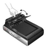
3. Wipe the feed roller from side to side. Rotate the roller to clean its entire surface.
