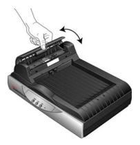
3. Slide the locking tab on the bottom of the scanner to its unlocked position. The scanner will not scan when locked.
