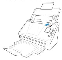
2. Locate the roller cover in the body of the scanner.
