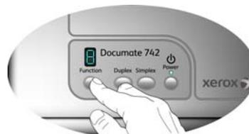
Press the **Function** button to cycle through the 9 One Touch scanning options
