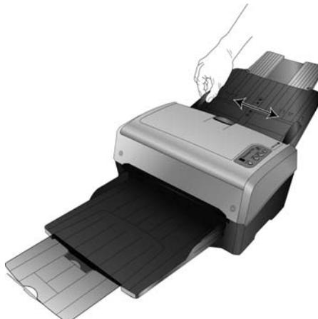
3. Load the documents *face down* with the top of the pages inserted into the Automatic Document Feeder.
