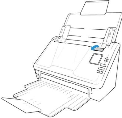
When you are done replacing the rollers, close the scanner carefully pressing down on both sides of the cover until it locks in place. Do not slam down the cover.
