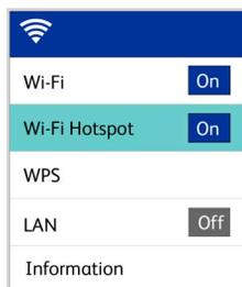
4. Navigate to **Information** and select it, then select **Wi-Fi**, then press down button to view the Hotspot IP and SSID.
