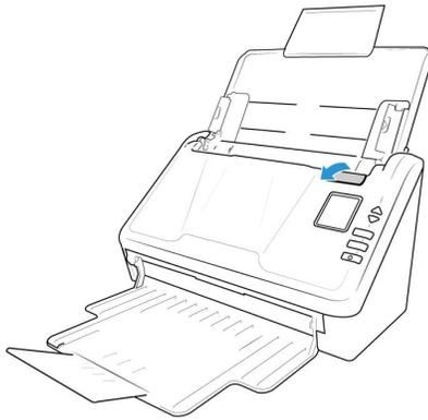
2. Locate the roller cover in the body of the scanner.
