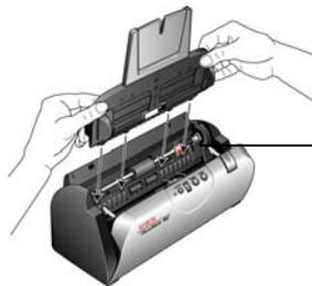
The roller is located in the body of the scanner behind the input tray.
