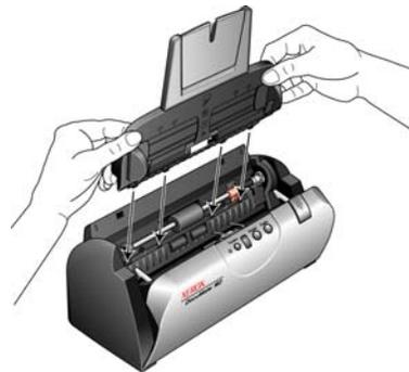
4. Push the paper guide back until it snaps into place. Close the scanner cover. Flip the paper guide extension up so it is fully extended.
