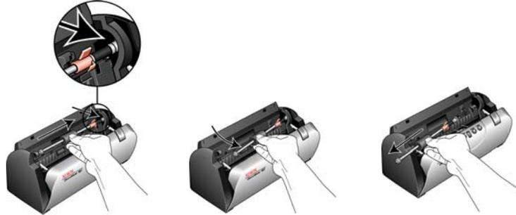
5. Discard the worn roller. It cannot be repaired.
