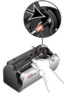
8. When you are certain that the gears are engaged, swing the roller into its scanner and align the left side with its mount. Then gently slide the roller to the left to fit its left end into its mount. Make sure the left end of the roller is firmly seated into its mount.
