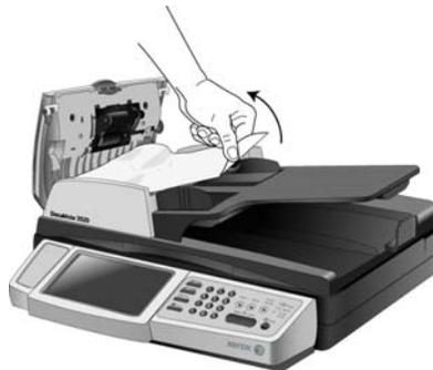
To reduce the number of paper jams, smooth and straighten paper before scanning, adjust the guides to the paper size, and insert the paper evenly into the ADF.
