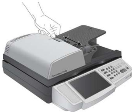
3. Adjust the Paper Stop at the back of the scanner for the length of the paper.
