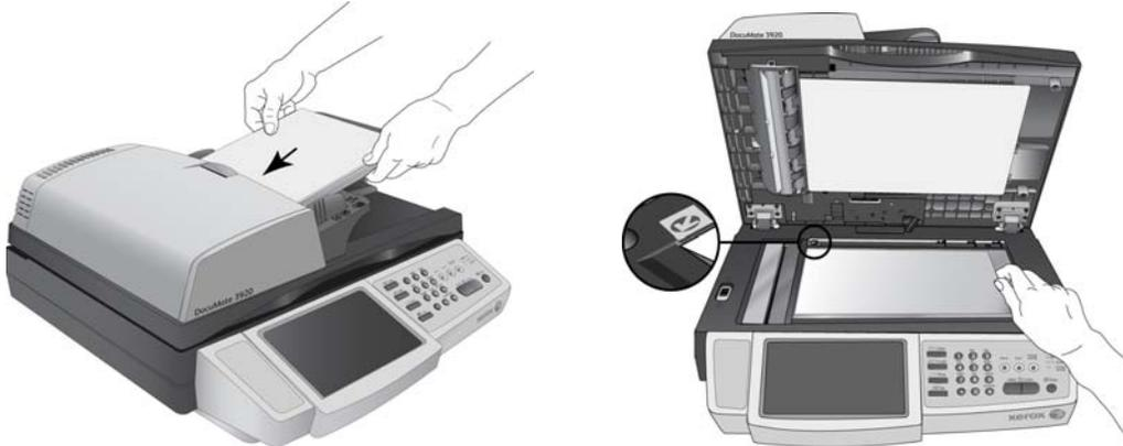
2. Press the Copy button on the scanner.
