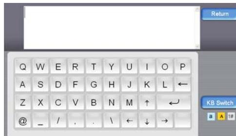
2. Press the **KB Switch** button to cycle through the keyboards 3 views (lower-case letters with common symbols, upper-case letters with common symbols, and number keypad with additional symbols).
