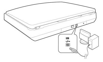
If the plug does not attach easily, make sure that you are plugging it in correctly. Do not force the plug into either connection.
