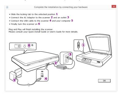
**Note:** If you do not see this on-screen diagram for connecting the scanner, stop and follow the instructions below.
