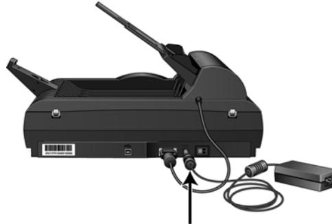
**NOTE:** Only use the power supply included with your scanner. Connecting any other type of power supply may damage your scanner, and will void its warranty.
