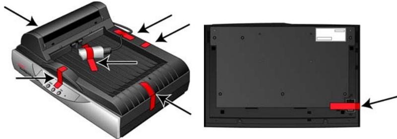
2. Open the ADF cover and carefully remove any foam particles that may have gotten inside the Automatic Document Feeder.
