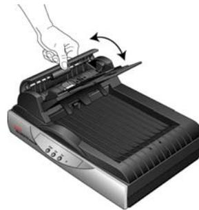
3. Wipe the feed roller from side to side. Rotate the roller to clean its entire surface.
