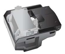
9. Pinch the arms on either side of the roller module and pull the roller module out of the housing.
