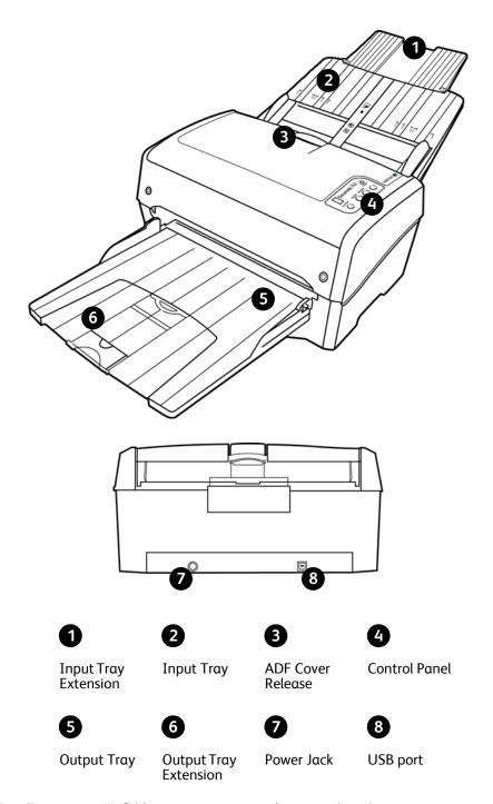
Input Tray Extension—Unfolds to support various document lengths.
