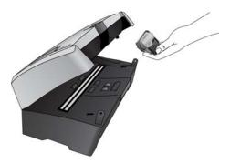
7. Place the roller housing face down on a flat surface.
