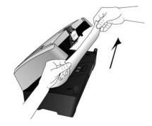
To reduce the number of paper jams, smooth and straighten the paper before scanning, adjust the guides to the paper size, and insert the paper evenly into the ADF
