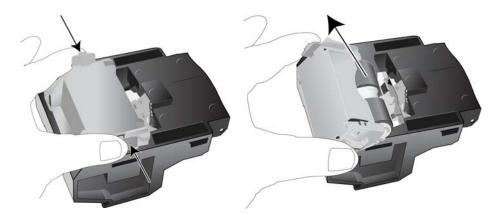
10. Place the new roller module in the housing a press down, on the back of the roller module, until the arms on the roller module snap into place.
