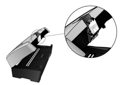
3. Place one hand on the ADF cover to hold the ADF cover open while removing the roller from the scanner.
