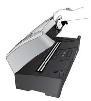
5. Firmly pull the roller housing towards you. You will hear it release from the scanner cover.
