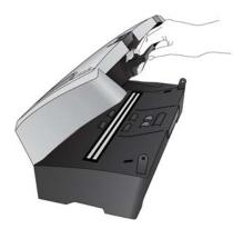
6. Leverage the roller housing out of the scanner.
