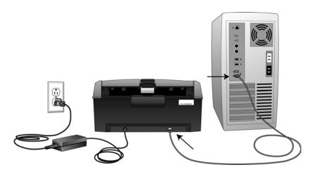
If the plug does not attach easily, make sure that you are plugging it in correctly. Do not force the plug into either connection.
