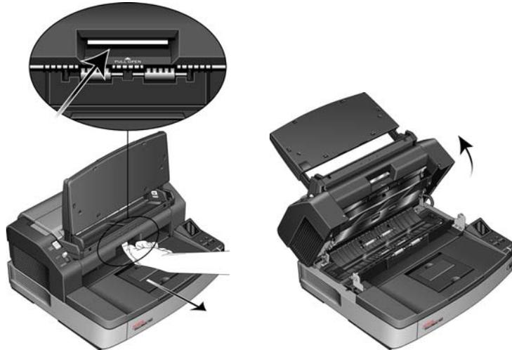
**NOTE:** Be careful when cleaning the rollers. All of the rollers, except the free rollers, are designed to rotate in one direction only. Do NOT force the roller to rotate in the opposite direction. Forcing the roller to rotate will damage it, and cause the scanner to feed pages incorrectly.
