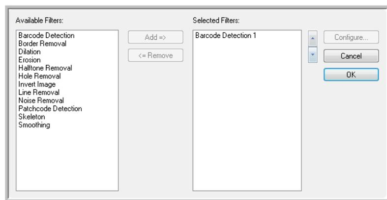
Click on a filter on the right side of the screen then click on the **<=Remove** button to remove it from the list.
