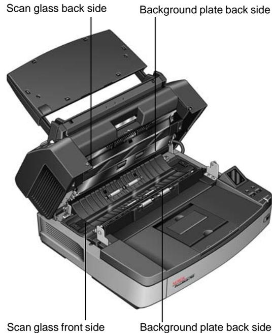
2. Wipe clean the glass and background plate in the underside of the exit door.
