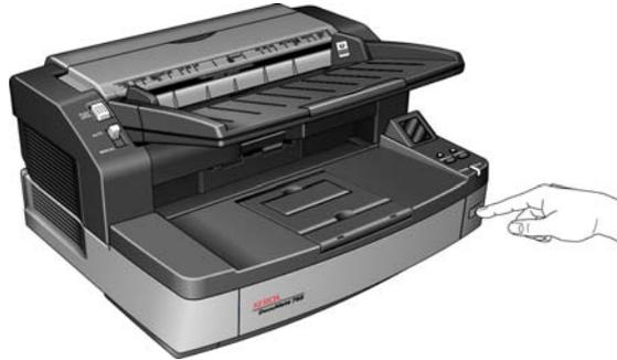
2. Using the blower brush, brush away any dust build up around the ventilation openings.
