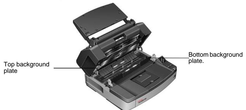
4. Place your left index finger on the outside of the bar top background and push inward against the spring. Keeping the bar pushed in, use your right hand and rotate the bar forward to flip the background plate to the opposite color.
