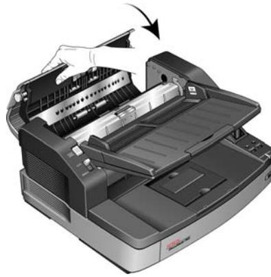
**NOTE:** If only the bottom of the page is visible, leave the ADF door open and follow the instructions below for removing the page from the exit path.
