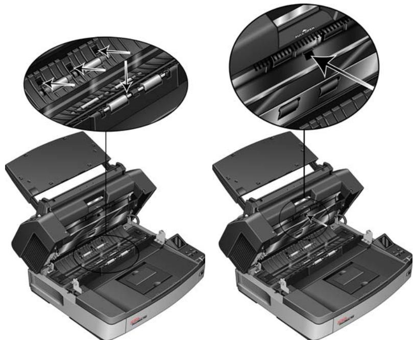
3. Point the tip of the blower at the sensor and squeeze the blower to direct a puff of air at the sensor head to remove dust.
