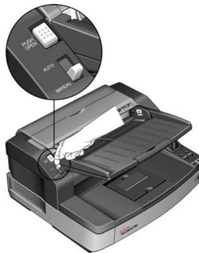
This drops the bottom feed roller away from top feeding rollers, making it easier to scan thicker pages through the ADF.
