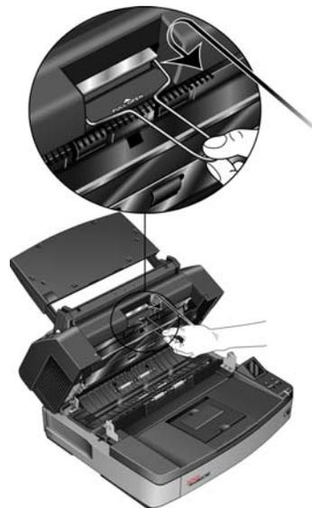
4. Close the scanner by carefully lowering the door to the scanner base until it is securely locked. Do not slam down the door.
