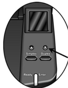
3. Press the **Simplex** button to scan a one-sided document. Press the **Duplex** button to scan a two-sided document.
