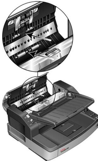
5. Wipe the Free rollers from side to side. Rotate the rollers downward to clean the entire surface of each roller.
