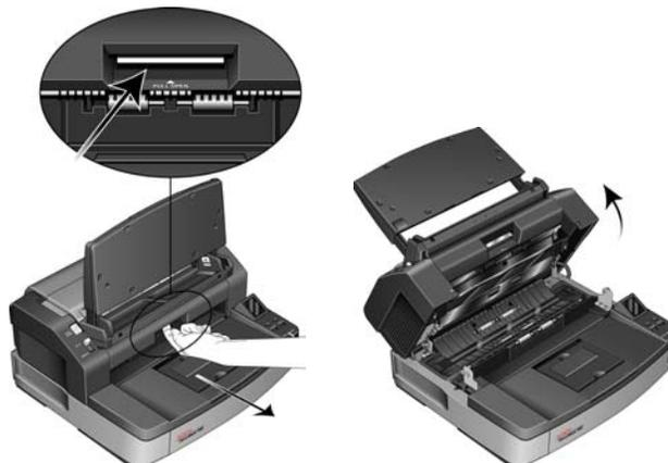
2. Locate the exit door release and hook the wire frame in the slot of the exit door release.
