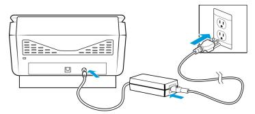
Xerox<sup>®</sup> FD70 Scanner Scanner Scanner Scanner Setup
