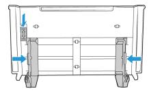
When the paper guide switch is in the down position, the paper guides can be adjusted to a maximum of 8.5 inches (216 mm) wide. If the paper guides are adjusted wider than the maximum for regular paper, documents may skew excessively during scanning.
