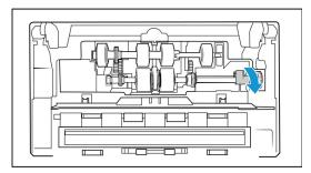
6. Carefully angle the roller up and out of the scanner and then discard it, it cannot be replaced.
