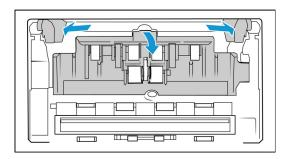
4. Rotate the belt upwards.
