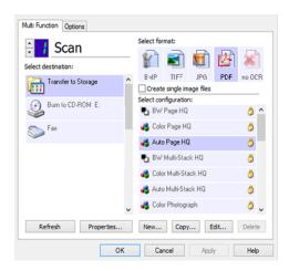
• **TWAIN and WIA Interface**—This option uses your scanner's TWAIN interface to scan. Select scanning options before scanning, put the document in the scanner, then click the **Scan** button in the TWAIN interface window.
