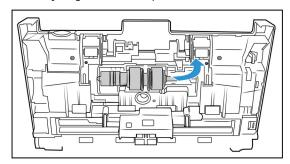
5. Remove the replaceable roller from the bar.
