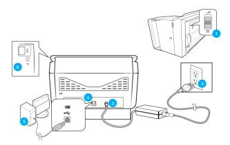
**Note:** If you do not see this on-screen diagram for connecting the scanner, stop and follow the instructions below.
