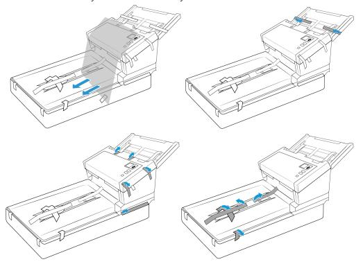
6. Open the automatic document feeder cover and remove any tape or protective foam from inside the feeder. Close the feeder cover when you are finished.
