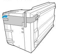
3. Remove the tape and slide the locking tab on the bottom of the scanner to its unlocked position. The scanner will not scan when locked.
