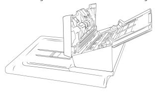
Use a soft cloth to wipe clean the glass. You can use a roller cleaning paper to clean the glass plates if there is any sticky residue on the surface.
