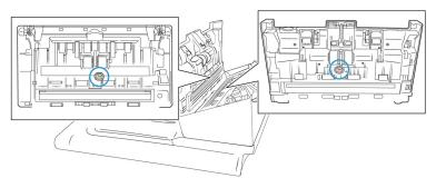
Using a clean, dry cotton swab, brush away any dust on the double feed detection sensors.
