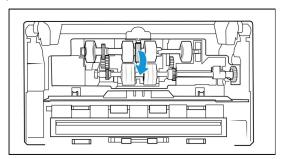
11. Lift the roller cover and carefully push it closed to lock it in place. Make sure everything is aligned properly and the cover is fully closed. If the cover is not fully closed it will break during scanning and damage the scanner.
