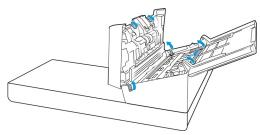
7. Lift the scanner lid. Remove any tape and protective foam from around or on the flatbed glass.
