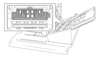
3. Move the paper guides to the side and then pull the feed roller cover away from the scanner.
