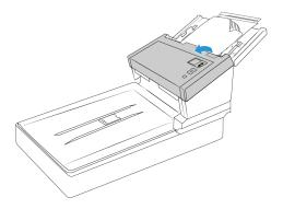
2. Locate and open the roller cover in the body of the scanner.
