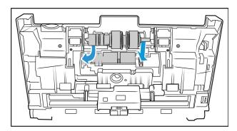
10. Lift the roller cover and carefully push it closed to lock it in place. Make sure everything is aligned properly and the cover is fully closed. If the cover is not fully closed it will break during scanning and damage the scanner.
