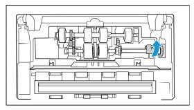
10. Rotate the belt back down into place. The cover will not close if the belt is in the wrong position.
