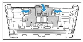
4. Carefully angle the roller up and out of the scanner.
