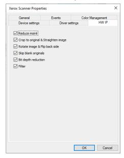
Click the check box to deselect (disable) hardware image processing only for the option listed. When one of the options in this window is not selected, software Visioneer Acuity will be used to perform that function while scanning.
