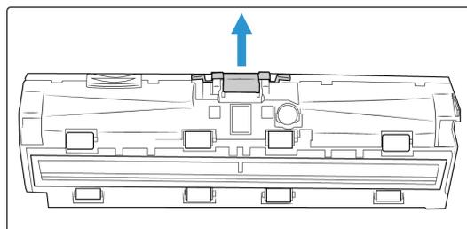
5. Coloque a nova almofada do ADF no scanner.
